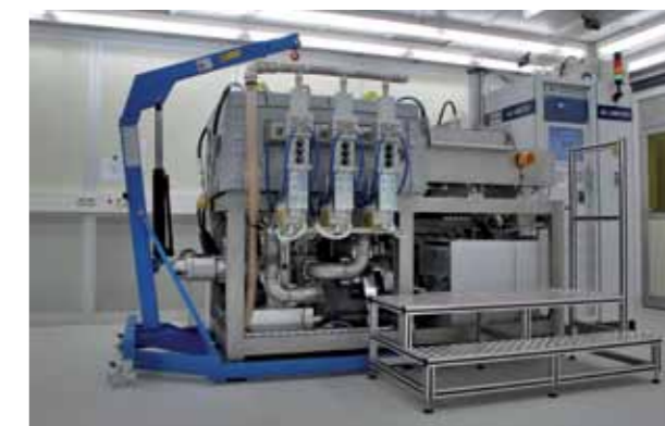
Fig. 1: Our new versatile usable plasma etch tool – a Roth & Rau Microsystems AK 1000 RIE.
