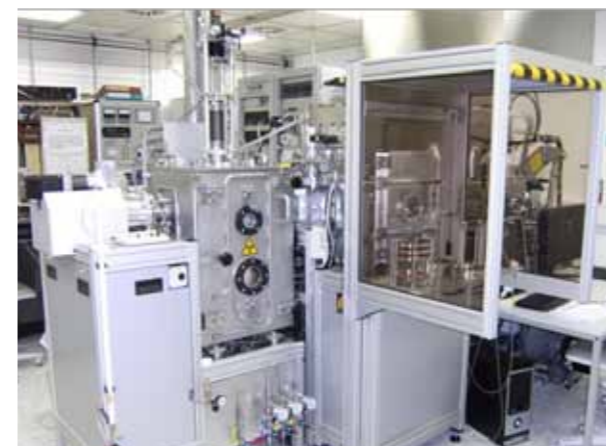
Fig. 1: Equipment for Electron Beam Evaporation and Sputter Deposition
